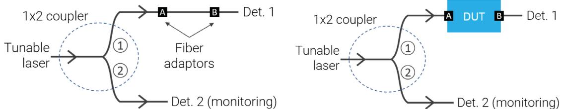
Figure 2. Two-step testing procedure.
