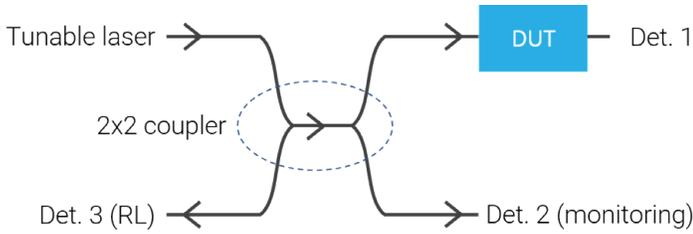
Figure 8. Typical IL and RL measurement setup.
