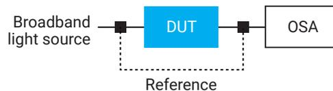
Figure 4. Typical configuration for IL measurement using a broadband light source and an OSA.
